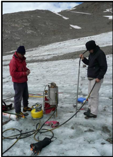
Pointwise mass balance measurements © E. Thibert, INRAE.
